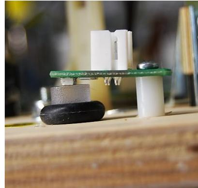
Save the #8 x 1/2" SMSs (shown in the photo below; we'll refer to these screws as <sup>44</sup> from now on) used to fasten the old brackets to the playfield; we will reuse them later. Your brackets may have a washer under them; the washers were used as a bracket spacer on very early WOZ builds. There is no need to keep the washers; they will **NOT** be used in the new bd installation process.
