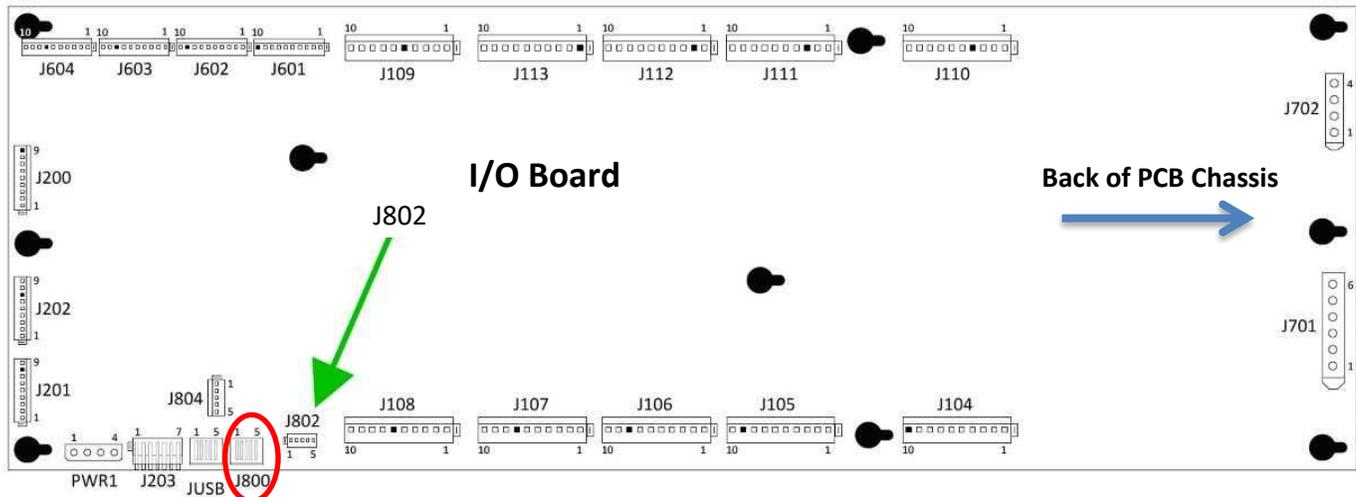
Locate the USB cable connected to J800 (circled in red above) on the I/O bd. Follow one of the two steps below:
