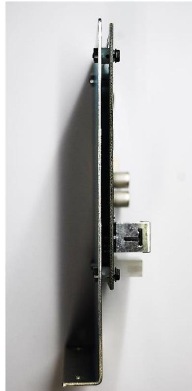
16) Using a ¼" nutdriver and two #8 x ½" SMSs <sup>44</sup>, attach the BAG bd <sup>13</sup>/mounting bracket <sup>2</sup> assembly to the underside, center of the playfield. Orient the bd and bracket as shown in the photos below (mark and predrill pilot holes).
