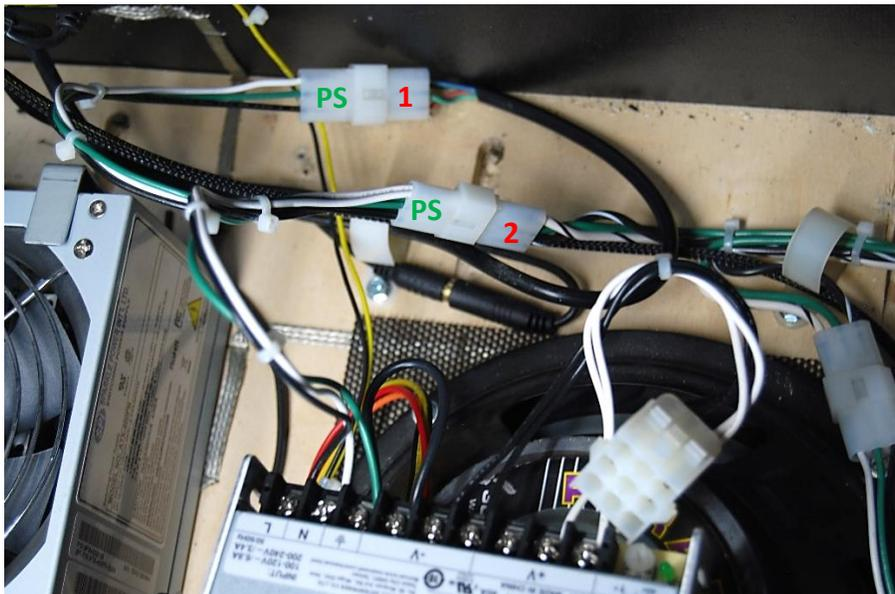
Using a ¼" magnetic nutdriver and two #8 x ½" SMSs <sup>44</sup>, attach the new power supply (by way of the two L brackets you installed earlier) to the bottom and back wall (or just the back wall) of the lower cabinet (mark and predrill pilot holes).
