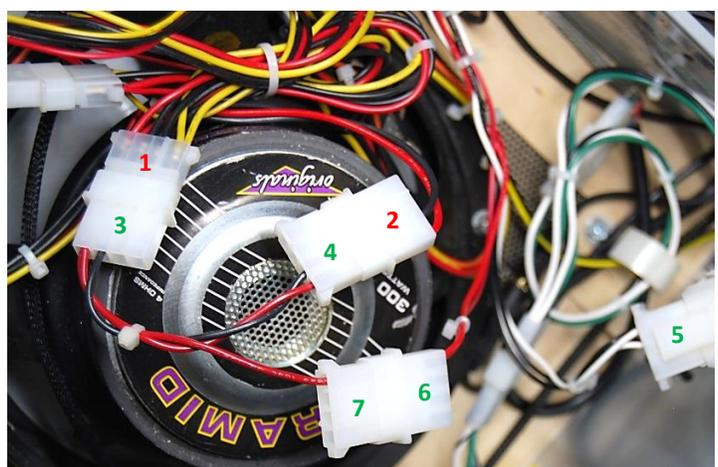
22) Cable tie <sup>36</sup> the new RGB power harness <sup>30</sup> and the shielded, 6-ft USB 2.0A to Mini-B cable <sup>29</sup> that you connected to the back of the CPU bd into the bundle running up to the playfield and fold them inside the black, corrugated, split tubing that protects the bundle.
